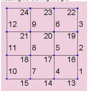
requires 24 wires. Each side of each square is a separate wire.
