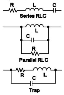
The load number column and specified and actual position columns function the same as for the <u>Sources Window</u>. Values of R, L, and C are entered in the appropriate columns. **EZNEC** will calculate and use the impedance of the RLC combination as required.
