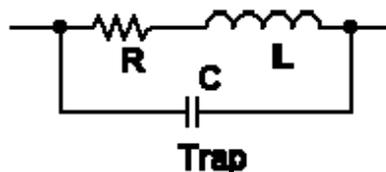
The load number column and specified and actual position columns function the same as for the [Sources Window](#). Values of R, L, and C are entered in the appropriate columns. **EZNEC** will calculate and use the impedance of the RLC combination as required.
