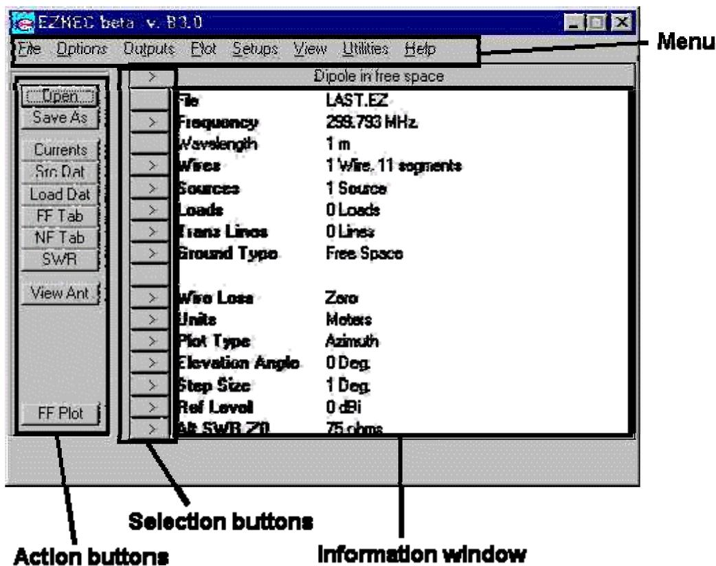
**Information Window** – This window shows information about a number of important parameters of the antenna being modeled. Any of the information in this window which can be changed is saved with the antenna description in the antenna description file.
