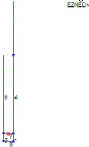
If it's necessary to test whether alignment is necessary in a particular situation, change the segmentation of one of the wires so that the segment junction alignment changes, and note the change in results. If the change is significant, segment alignment is important.
